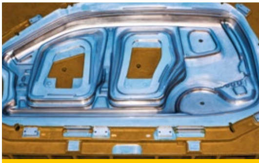
PKW-Seitenwandmatritze aus GGG 70L A car side panel moulding made of ductile cast iron 70L
